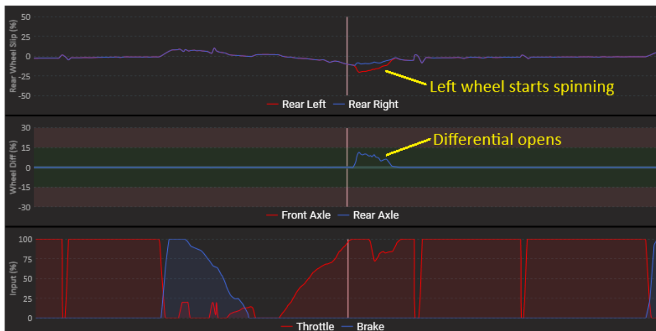
Figure 3.21: High Power Ramp Angle (Low Locking Effect)
