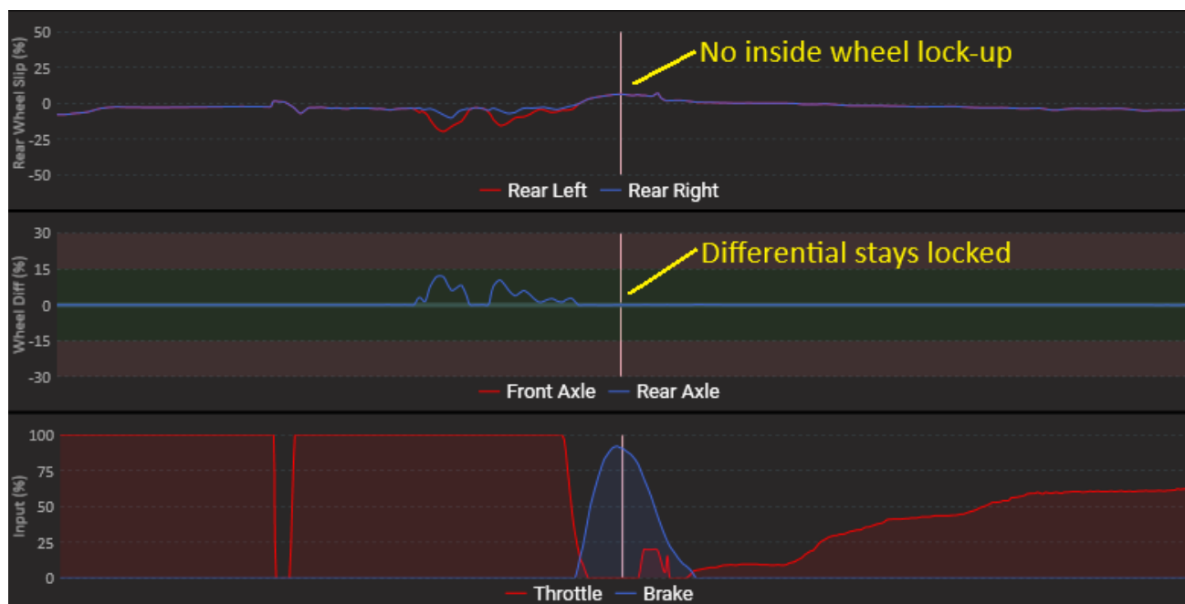
Figure 3.24: Low Coast Ramp Angle (High Locking Effect)
