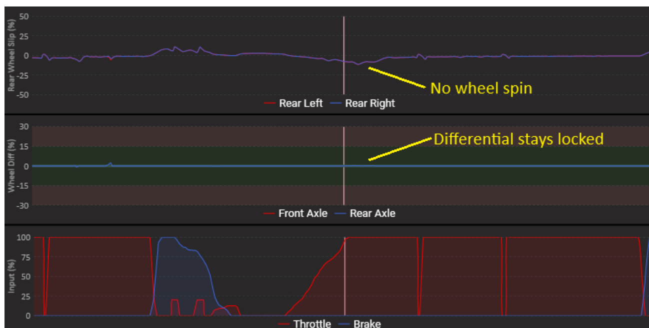
Figure 3.22: Low Power Ramp Angle (High Locking Effect)
